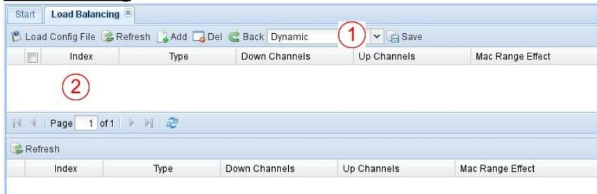
1. General LoadBalancingconfiguration - the most typical configuration is “Dynamic”
